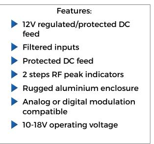
The AS-122 allows you to optimise your RF coverage in your bag or your cart. You can use passive antennas and compensate loss in cable thanks to the DC-feed supply, distribute RF signals up to 6 diversity receivers.
